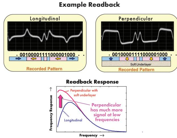
**Figure 5: The readback waveforms change dramatically between longitudinal and perpendicular recording. The signal processing in the R/W channel must be able to accommodate these new waveforms and appropriately include some of the extra signal energy available at low frequencies.**
